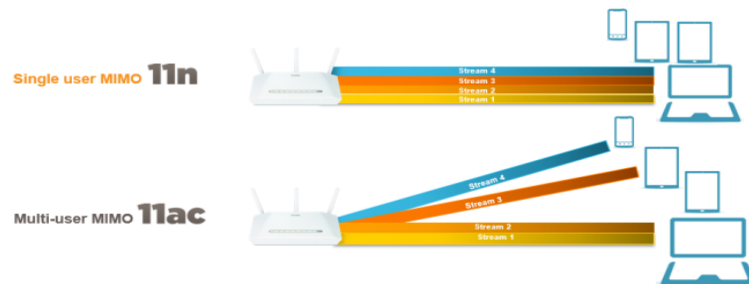
Figure 2. SU-MIMO and MU-MIMO operation
