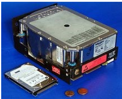
A newer 2.5-inch (63.5 mm) 6,495 MB HDD compared to an older 5.25-inch full-height 110 MB HDD
